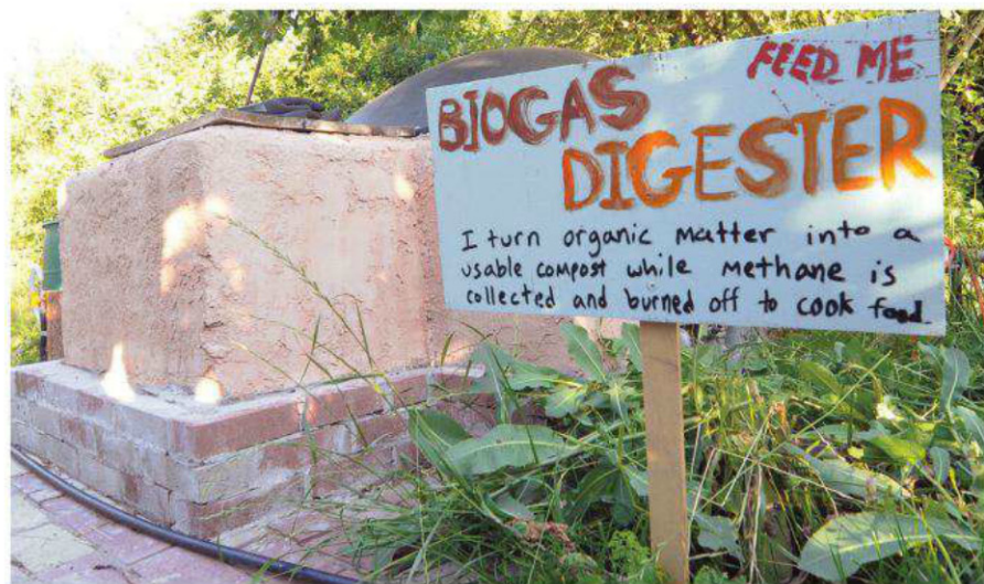
A 200-gallon generator in Oregon turns 15 pounds of food waste into cooking fuel daily.
